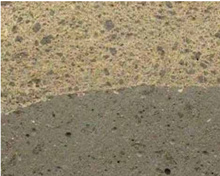
Figure 9. Cut surface of a 60% alumina colloidal silica material cast onto a 75% alumina-15% SiC product and fired to 1500°F.
